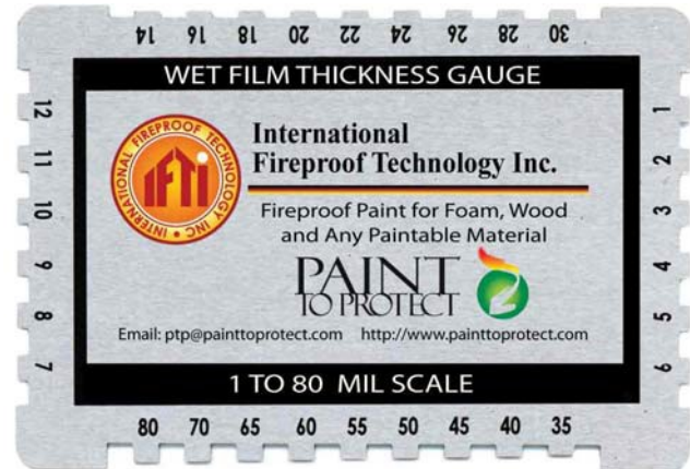
Figure 1. Notch Type Wet Film gauge
