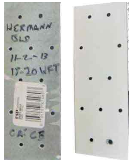
Figure 3. Front and back of Medallions. These mending plates can be purchased at local hardware stores.
