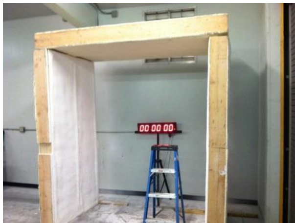
Test Set up for Ceiling Assemblies
